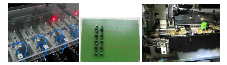
Tooling to accommodate a variety of applications-field reconfigurableSingle Span: 2.5mmDual Span: 2.5mm/5.0mmTriple Span: 2.5mm/5.0mm/7.5mm
